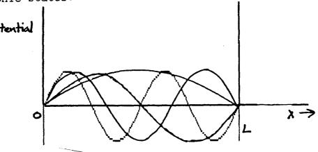
Some electron waves that may be confined in potential well of width L
