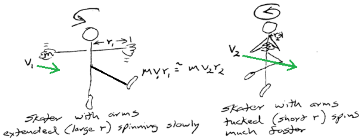
Figure 1.17. Rate of spin increases when spin radius decreases (instantaneous velocity v_2 greater than v_1 ).
