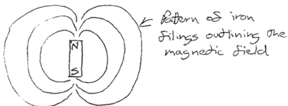
Figure 1.20. Pattern of iron filings sprinkled around a bar magnet.
