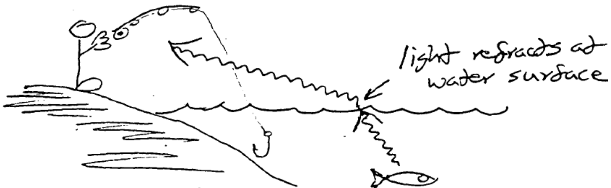
Figure 2.1. Refraction of light at the water's surface. To the fisherman, it would appear the fish was farther away from shore, along the beam of light coming to his eyes from the water surface.
