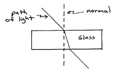
Conversely, when light passes from glass to air, it bends away from the normal. Trace the paths of light beams through the bi-convex lens illustrated below to show how astronomers
