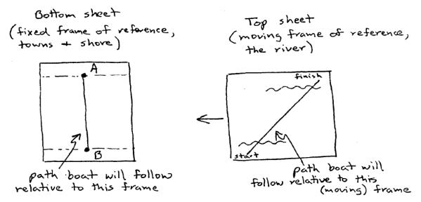
Attach a 12 inch string to its bumper and place the car on the plastic "river" (imagine the car is a boat). Pull it on a diagonal across the "river" so that, as the river "current" flows past the towns, the car rolls on a straight line (relative to the fixed paper frame) between A and B. With some practice, you can demonstrate that the "boat" must traverse a longer (diagonal) path on the frame of reference of the river in order to cross directly between the two towns.
