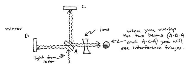
Put the apparatus on a cart, and reproduce the Michelson-Morley experiment: do you see any change in the interference pattern as you rotate the cart relative to the presumed "ether current?"
