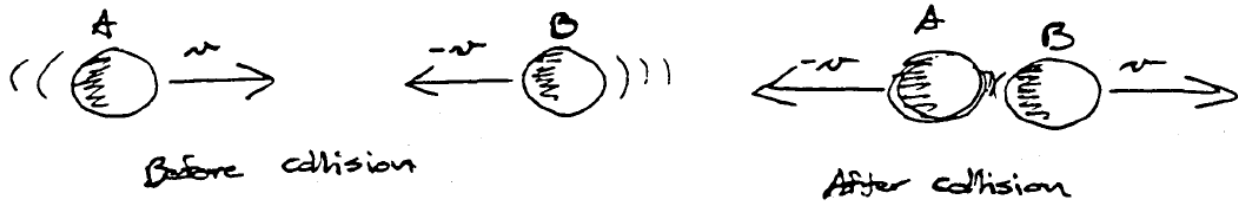
Figure 3.7. Conservation of momentum in a collision between two billiard balls with equal mass.
