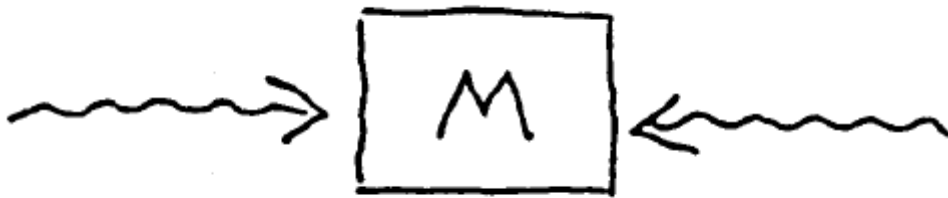
Figure 3.11. Mass absorbing two photons of equal but opposite momentum.
