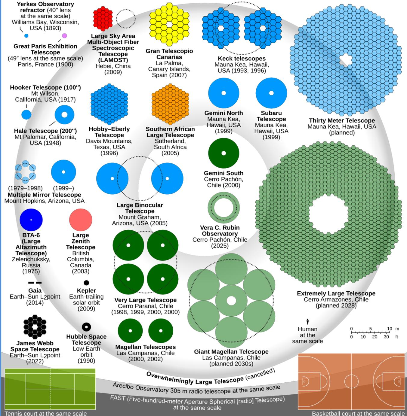
A sampling of the world's optical telescopes. Note latest segmented design with adaptive optics.
