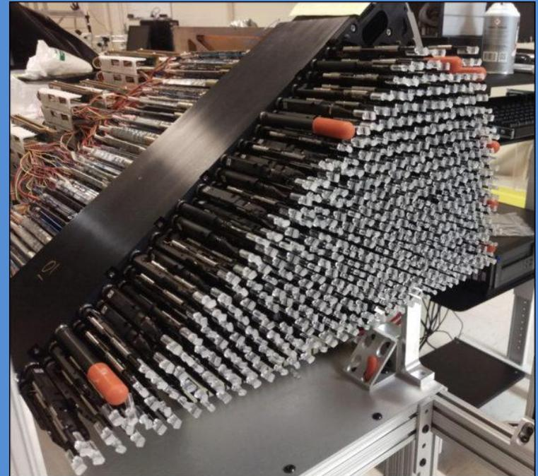
Focal plane robots at DESI collect spectra from 5000 objects at once.
